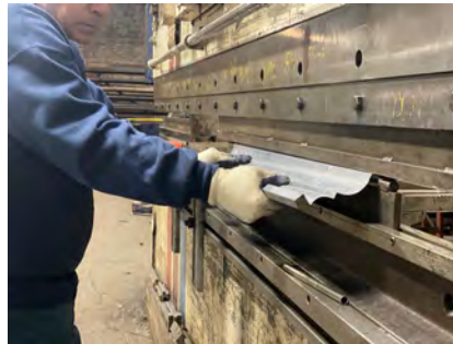
Worker at a metal machine shop in Northeast Philadelphia uses a "brake" to shape metal to match deteriorated trim that was pulled off the building.
