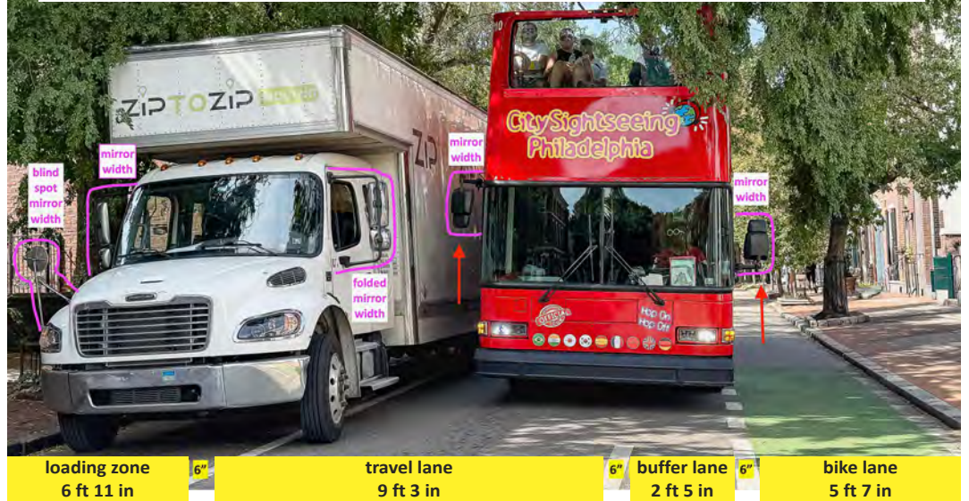
Commercial vehicles are typically 8 feet 6 inches wide with 12-15 inch mirror spans on each side, resulting in an effective width of more than 10 feet.
