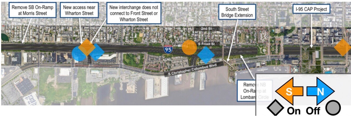
Figure 3 I-95 Access Points for the Medium Impact Design Concept (Market Street to Morris Street) base source: PennDOT
