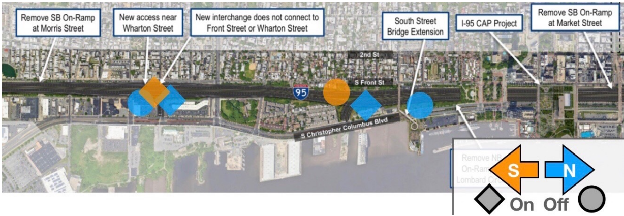
Figure 4 I-95 Access Points for the High Impact Design Concept (Market Street to Morris Street) base source: PennDOT
