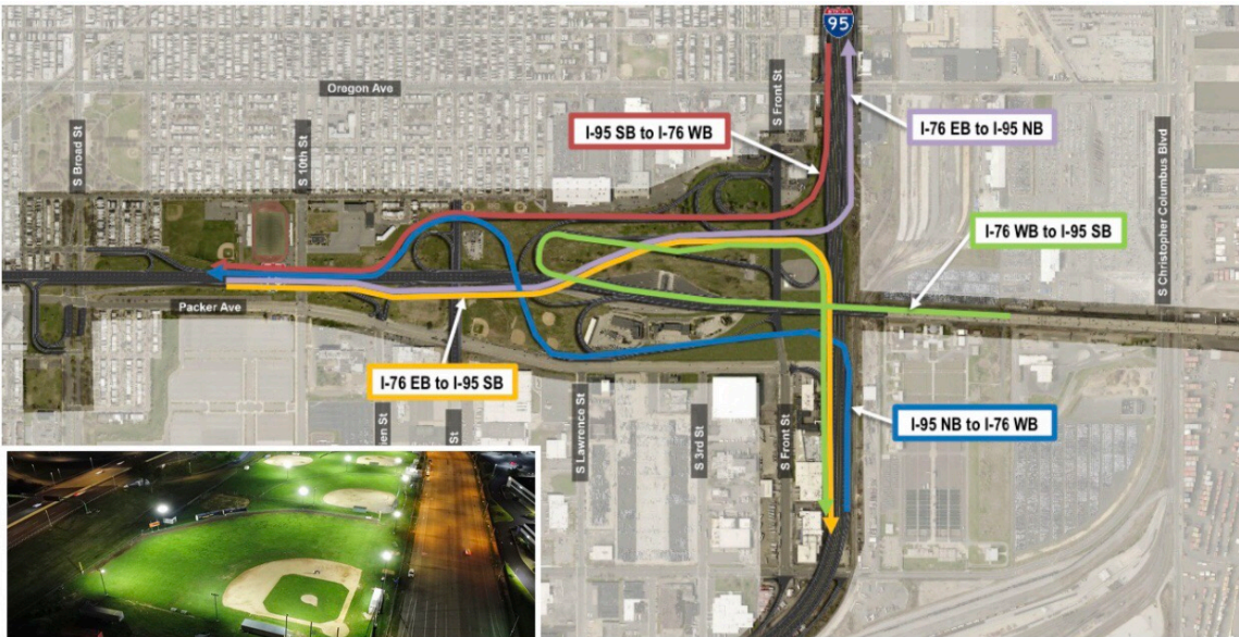
Figure 9 PennDOT Low/Medium Impact Design Concept for Walt Whitman Interchange base source: PennDOT; ballfields inset: Mark Kapczynski
