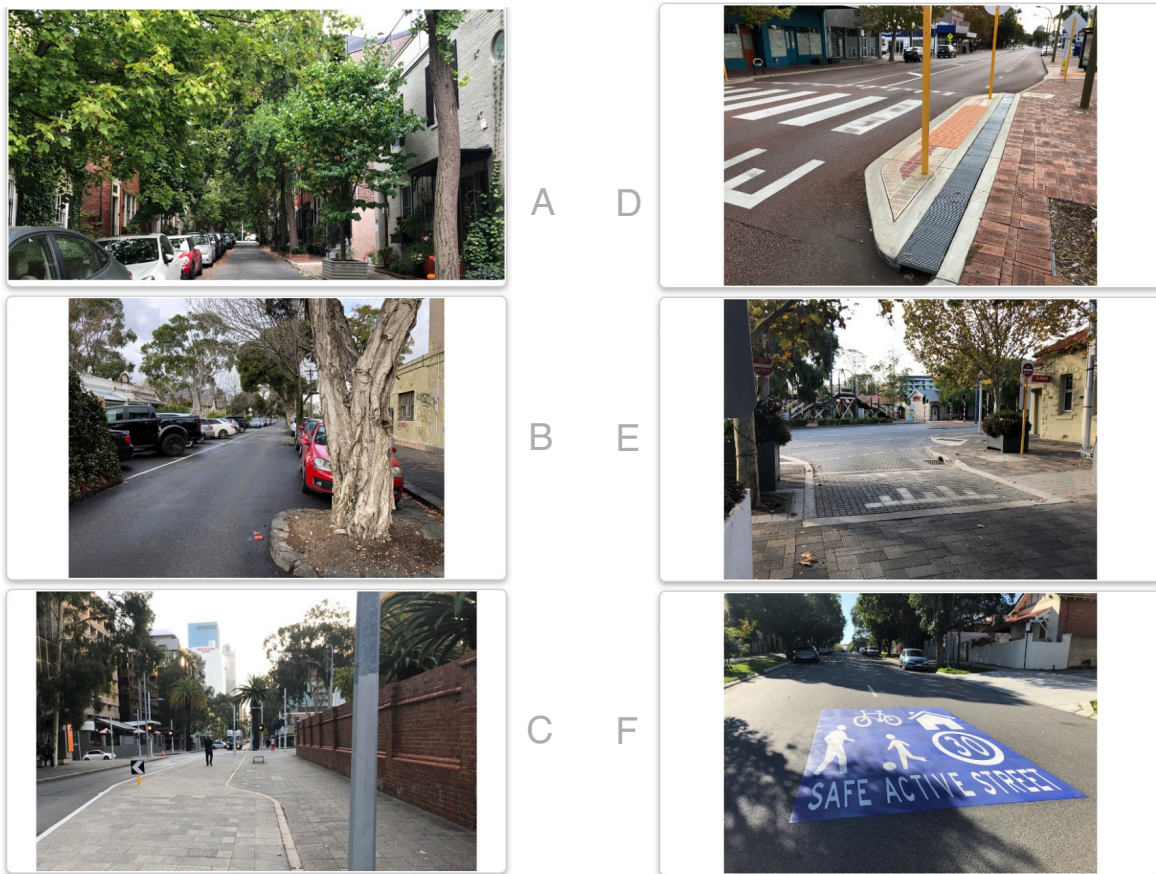
Figure 15 Examples of Traffic-Calming Treatments
